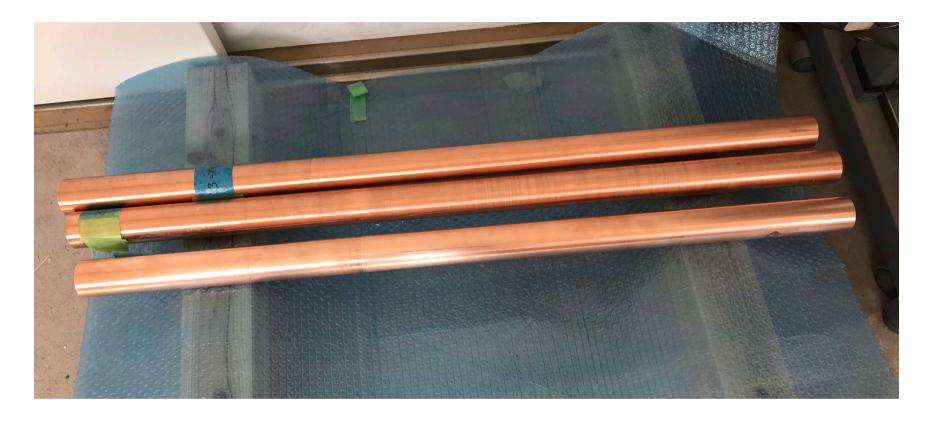
Cu-Ag rod made from casting material by forging, heat treatment and machining surface. This rod will be drawn to obtain the 2mm  $\times$  3mm rectangular wire.
