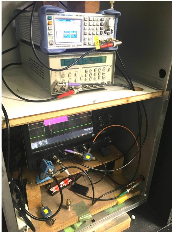
The setup for the RF measurement
